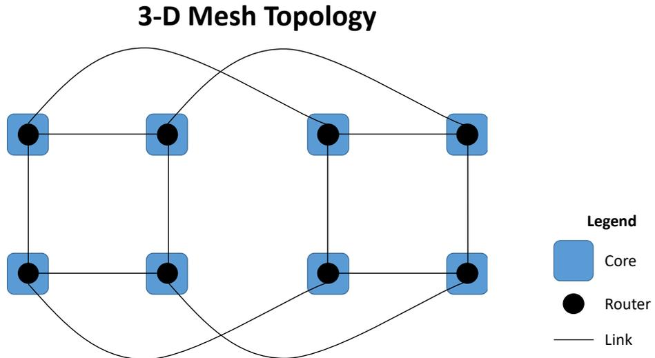
The above diagram shows a 3-D mesh with  $N=8$  nodes. For a system of  $N$  nodes, the 3-D mesh topology consists of  $k = N^{1/3}$  nodes in each dimension.
