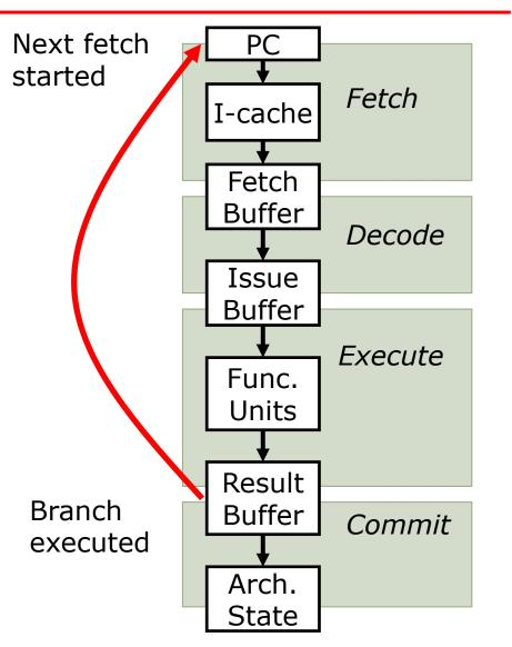
Modern processors may have > 10 pipeline stages between next PC calculation and branch resolution!
