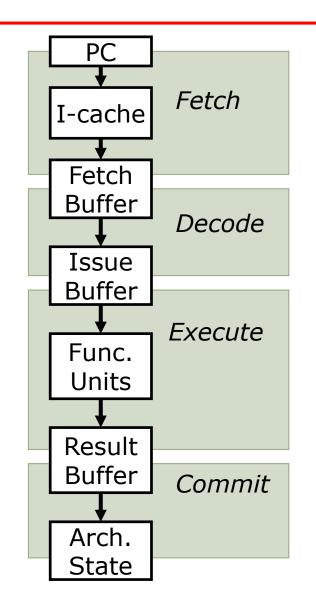
Modern processors may have > 10 pipeline stages between next PC calculation and branch resolution!
