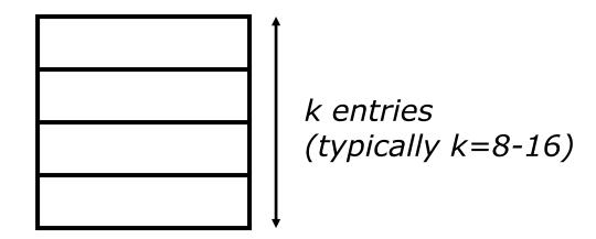
Small structure to accelerate JR for subroutine returns, typically much more accurate than BTBs.
