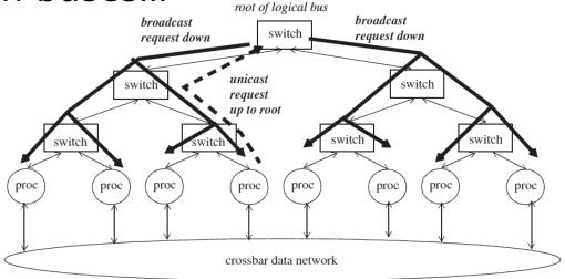
Starfire E10000 (drawn with only eight processors for clarity). A coherence request is *unicast* up to the root, where it is serialized, before being *broadcast* down to all processors
