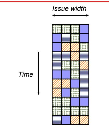
• Interleave multiple threads to multiple issue slots with no restrictions
