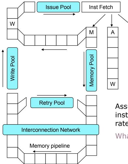
• Every cycle, one instruction from one active thread is launched into pipeline
