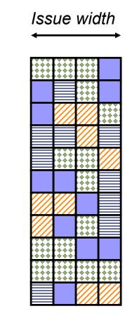
For regions with low thread level parallelism (TLP) entire machine width is available for instruction level parallelism (ILP)
