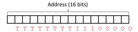
Divide the bits of the address according to how they are used to access the cache (tag, index, offset). Drawn above (letters). Block size is 32 bytes, so there are five offset bits. We have 8 lines in a direct mapped organization (as indicated by diagram), so we need three index bits. The remaining 8 bits constitute the tag.
