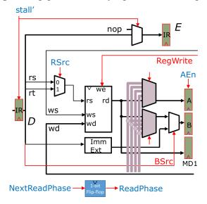
Alyssa notices that bypassing can avoid some stalls for instructions that use two source registers: if at least one of the source operands is available in a bypass path, then the single read port can be used to read the other operand, and decode does not need to stall!
