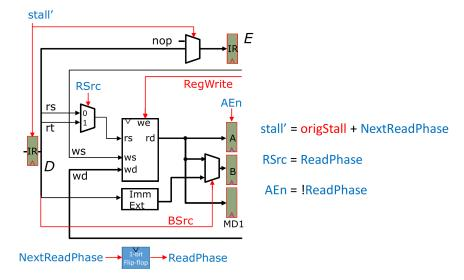
This design works as follows: if the instruction reads two source registers, then decode takes two cycles to resolve the structural hazard on the register file:
