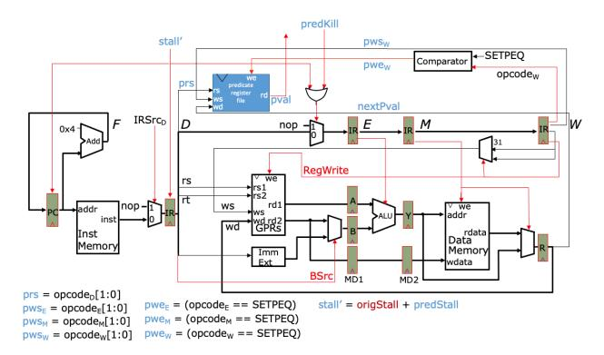
**Every predicated instruction and SETPEQ has its source/destination predicate register address encoded in the bottom two bits of its opcode**. When a predicated instruction enters the decode stage, it uses *prs* to select the predicate register to read. The register file outputs *pval*, which is the corresponding predicate register value. Predicated instructions must be treated as no-ops if the predicate register value is 0. To do this, Ben implements a new kill condition *predKill*.
