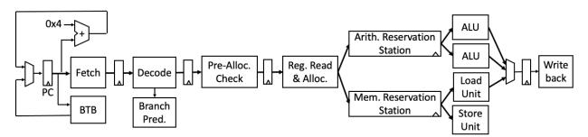
Figure 1: Simplified out-of-order pipeline schematic. Several important structures are not shown, such as commit, bypassing, and some sources of next-PC value
