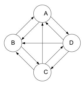
Note that each link is unidirectional, and only one link exists between A and C (only a link from C to A (not from A to C), and only from D to B between B and D. Each link can transfer 1 flit per cycle and there is only one virtual channel per link. For all parts, 180-degree turns are not allowed.
