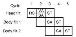
Consider the same scenario as in question 1, with packets A and B going to the same output unit. Assume that **non-speculative switch allocation requests are always prioritized over speculative ones** (i.e., those from flits without a VC). Fill in the following waterfall diagram to show how packet A is routed.
