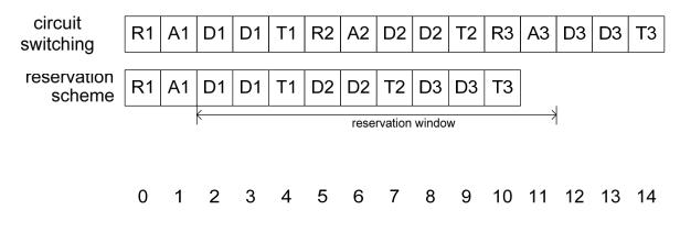
Note that tail flits may be able to get eliminated in this new scheme if they are used only to indicate when channels can be deallocated.
