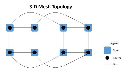
The above diagram shows a 3-D mesh with N=8 nodes. For a system of N nodes, the 3-D mesh topology consists of  $k = N^{1/3}$  nodes in each dimension.
