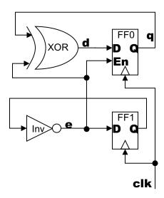
Draw a state transition diagram or fill out the state-transition table below for the sequential logic drawn above.
