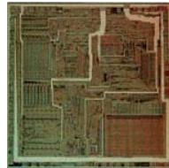
Intel 8086, 1978, 33mm 2 10Mhz, 29K transistors, 3u
