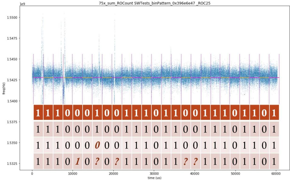
Figure 3: Example 60ms capture, recorded with 75 ROs, a integration period of 500ns, running a software victim. Expected data is shown in row 1 (white on red), extracted values by 3 untrained friends in rows 2-4.
