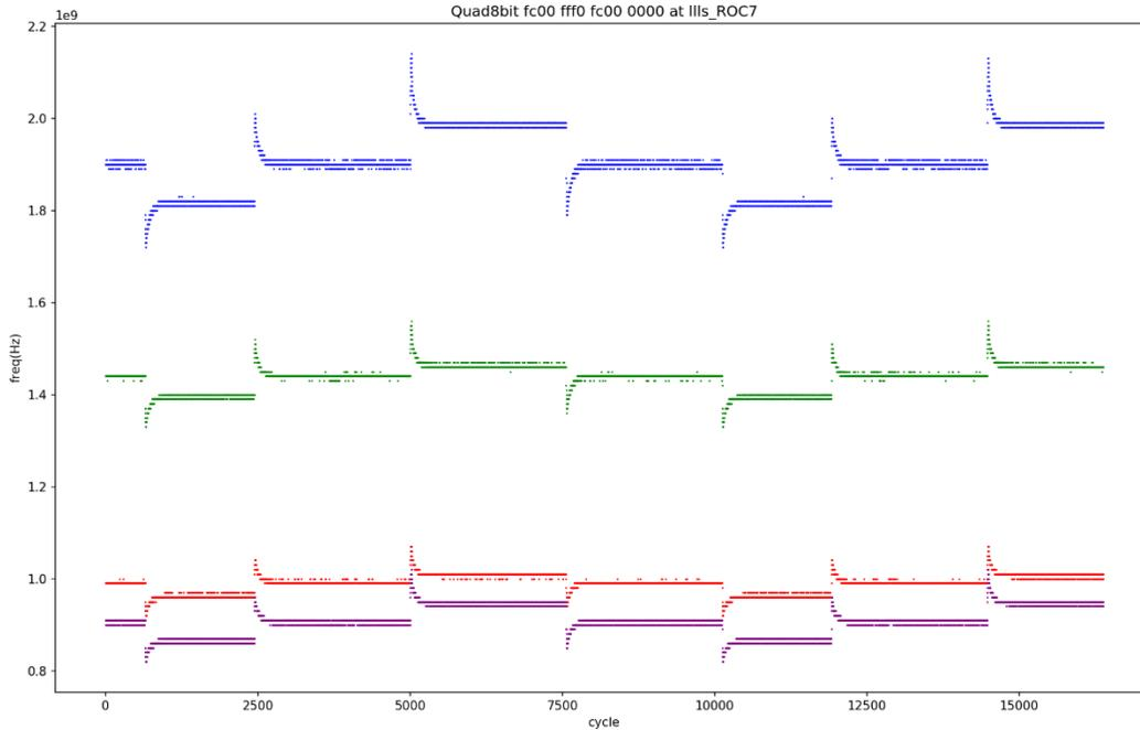
Figure 2: Frequency of 4 separate ROs recorded simultaneously, each "cycle" is 1 recorded sample, sampling at ~12MHz
