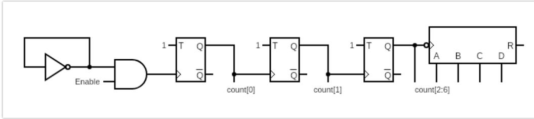
Figure 1: Ring Oscillator with 3 TFFs and 4+ bit counter
