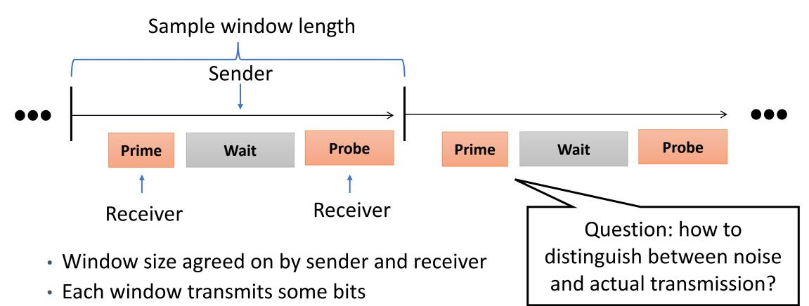
Sender & receiver need to perform an window alignment at the start
