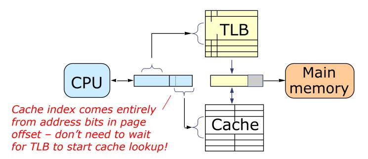
OBSERVATION: If cache index bits are a subset of page offset bits, tag access in a physical cache can be done *in parallel* with TLB access. Tag from cache is compared with physical page address from TLB to determine hit/miss.
