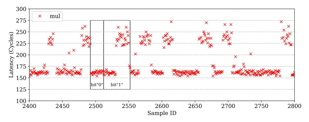
Access latencies measured in the probe operation in Prime+Probe. A sequence of "01010111011001" can be deduced as part of the exponent.
