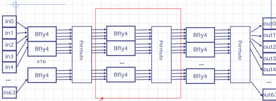
Reuse the same circuit three times to reduce area
