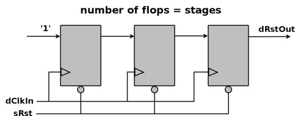
Figure 23: Module for synchronous resets
