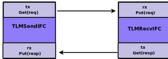
Figure 28: Connecting TLM Send And Receive Interfaces
