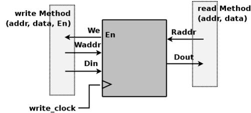
Figure 19: Asynchronous RAM
