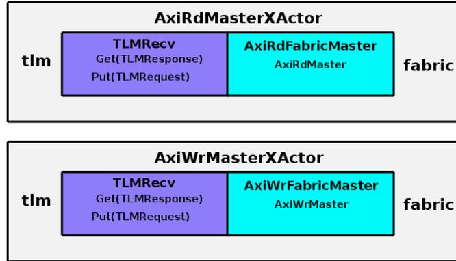
Figure 35: AXIMasterXActor Interfaces (Read and Write Versions)
