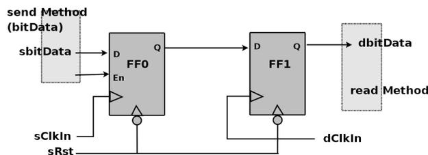
Figure 13: Bit Synchronizer 1.0 - single register in destination domain
