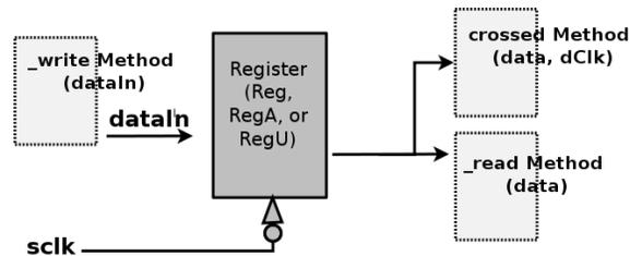
Figure 21: Register with wire synchronizer
