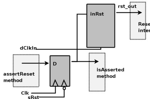
Figure 24: Module for generating resets
