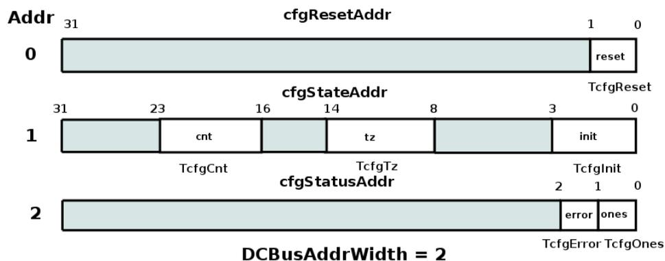
Figure 27: CBus Registers used in Block example
