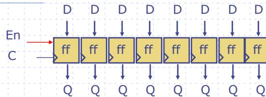
*Register:* A group of flip-flops with a common clock and enable
