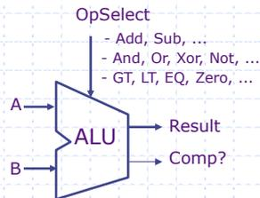
Such circuits have no cycles (feedback) or state elements
