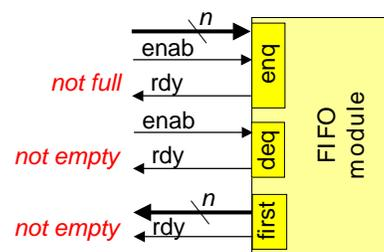
$n$  = # of bits needed to represent the values of type "a"
