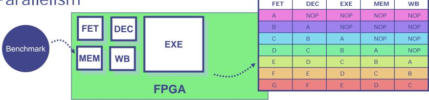
On one FPGA clock tick we will be simulating many different modules
