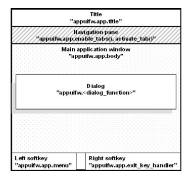
Figure 5.2: The different parts of the screen when using the 'normal' layout
