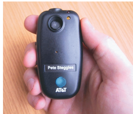
Figure 2. Bat wireless tag device. Powered by a single AA lithium cell, each Bat has a unique 48-bit ID, two input buttons, and—for output—a buzzer and two LEDs.
