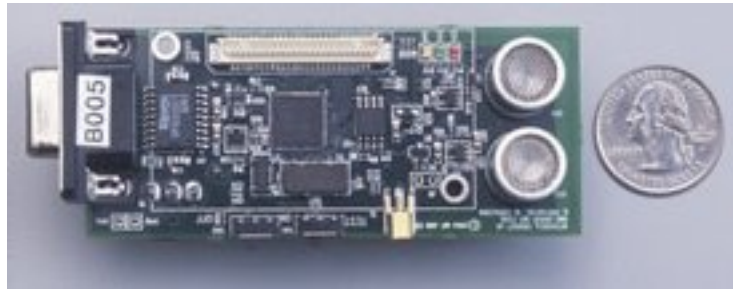
Figure 1-4: A Cricket hardware unit; this unit can function as either a beacon or a listener.
