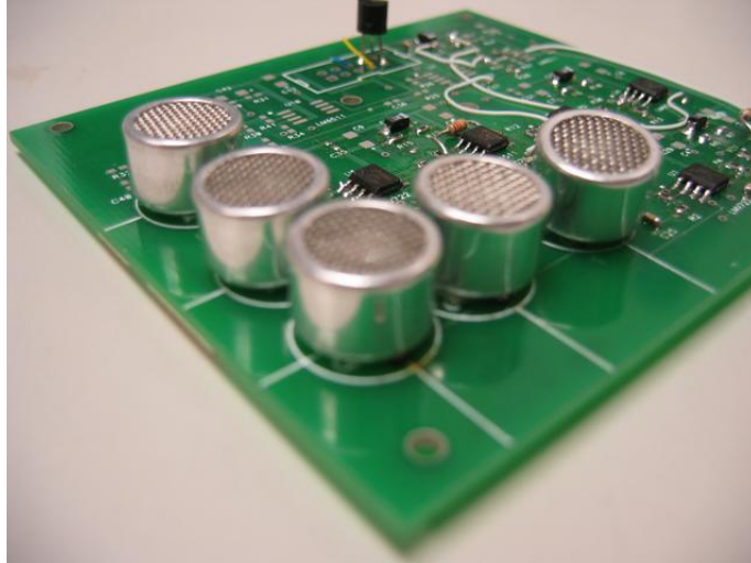
Figure 5-29: A Cricket compass board with five receivers arranged in two arrays of three receivers each.
