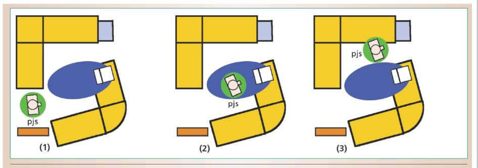
Figure A. Spatial monitoring application that moves users' desktops around with them. The application registers with the Spatial Monitor (1); as the user (pjs) approaches the display (2) or moves away from it (3), the spatial monitor sends a positive or negative containment event to the application that transfers or removes the desktop to or from the screen.
