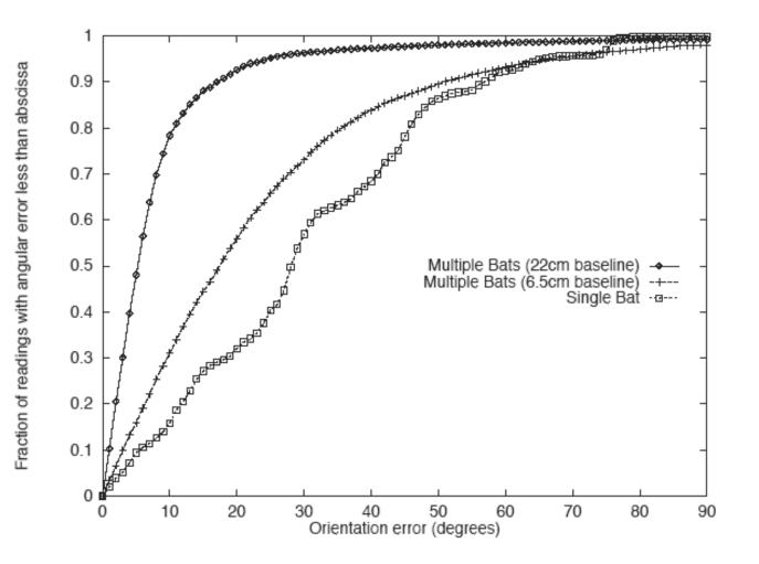
Figure 4. Orientation accuracy of ultrasonic tracker
