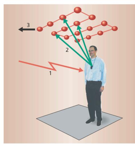
Figure 1. Operation of the Bat location sensor system. A Bat is triggered over a wireless link (1), which causes it to emit an ultrasonic pulse (2). Ceiling-mounted receivers measure the pulse's times of flight, and a controller retrieves the times of flight (3) over a wired network. The controller uses these measurements to calculate Bat-receiver distances and thus the Bat's 3D position.
