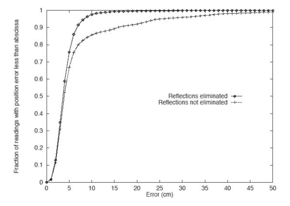
Figure 3. Position accuracy of ultrasonic tracker
