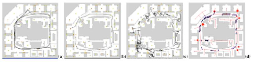
Figure 3: (a) Trajectory of the robot during a 25 minute period of training data collection. True path (in light color) and most likely path as estimated using (b) Voronoi tracking and (c) original particle filters. (d) Motion model learned using EM. The arrows indicate those transitions for which the probability is above 0.65. Places with high stopping probabilities are represented by disks. Thicker area and bigger disks indicate higher probabilities.
