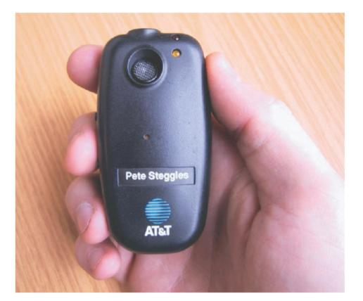
Figure 2. Bat wireless tag device. Powered by a single AA lithium cell, each Bat has a unique 48-bit ID, two input buttons, and—for output—a buzzer and two LEDs.
