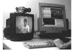
$\begin{tabular}{ll} Figure 3.2 & A typical configuration for an analog media space node, with a video camera, microphone, video monitor and workstation \\ \end{tabular}$
