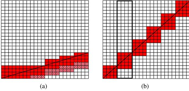
Fig. 5. **Cache Behavior at Varying Ray Angles:** Figure (a) shows an example of a cache with 4-word burst size. Shaded blocks are needed for ray computation, checked blocks are resident in the cache but will never be used again. Figure (b) shows the  $\frac{\pi}{4}$  case, in which all blocks in the cache are fully utilized. The dark box in Figure (b) is a column.
