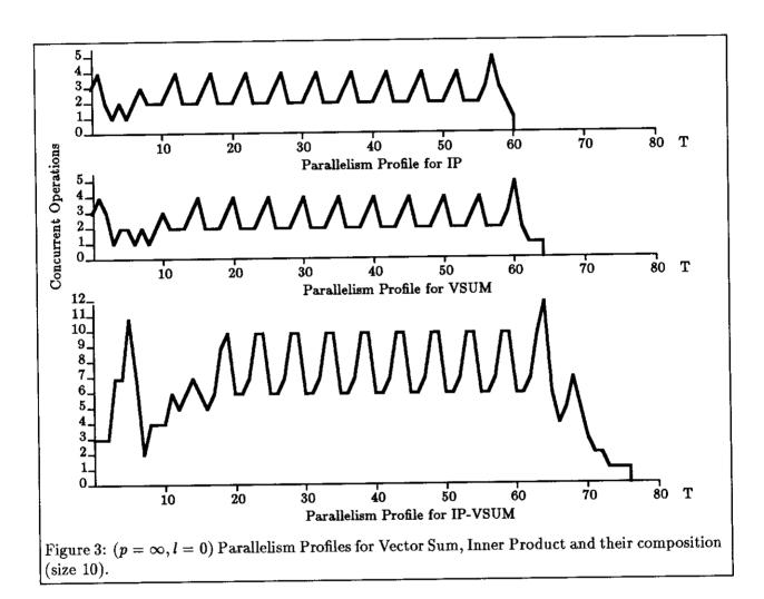
the inner-most loop is done sequentially. The rapid oscillations reflect the cumulative effect of the variations in parallelism in the inner-most loop. We could spawn the inner loops in a tree, and perform the summations as a binary tree to reduce the length of the critical path further, but it is evident that substantial parallelism is present even in the traditional algorithm.
