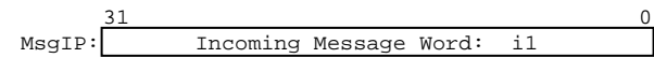
Figure 7: Hardware computation of MsgIp . Typically case 1 applies. If there are no exceptional conditions, neither queue is over its threshold, and the arrived message is of type 0, then case 2 applies.
