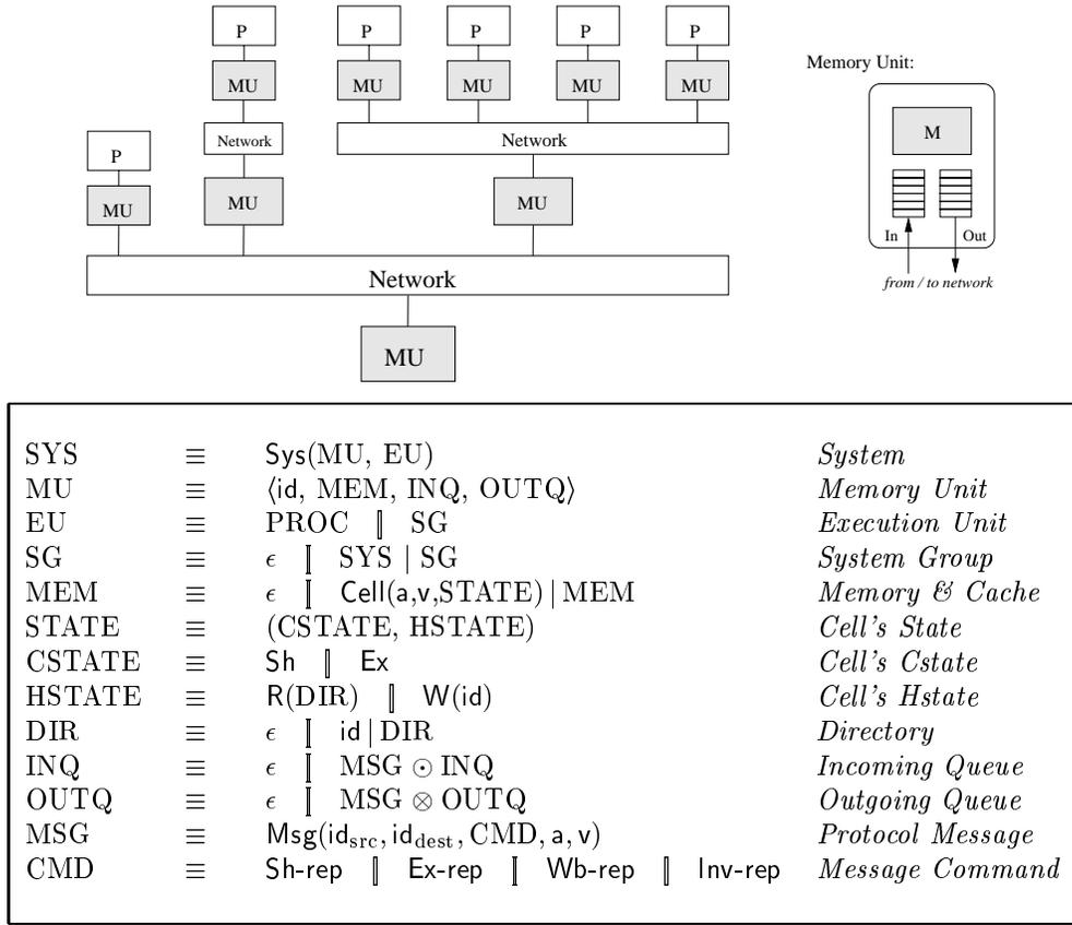
Figure 5: Grammar of the HCN Model (Initially, all non-outermost memories, and all incoming and outgoing message queues are empty; the outermost memory contains a cell in the  $(Ex, R(\epsilon))$  state for each address)
