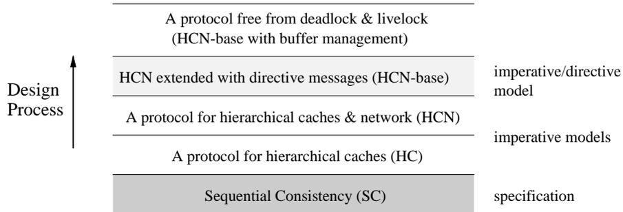
Figure 1: Design Process: Models to be Discussed (SC is the specification of Sequential Consistency, HC defines a protocol for systems with hierarchical caches, HCN is a refined version of HC with message passing, and HCN-base is a HCN-based cache coherence protocol that is free from deadlock and livelock)
