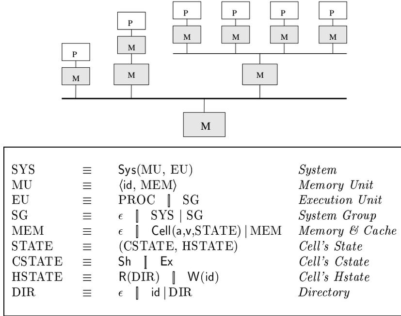
Figure 3: The HC Model (Initially, all memories except the outermost memory are empty; the outermost memory contains a cell for each address and the initial state of each cell is  $(\text{Ex}, \text{R}(\epsilon))$ )
