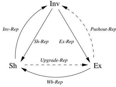
Figure 6: State Transitions Caused by Imperative Messages (Inv represents the state that the address is not cached in the memory; *Pushout-rep* and *Upgrade-rep* are potential optimizations for the HCN model)
