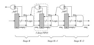
Figure 7: Synchronous pipeline with combinational multistage feedback flow control.
