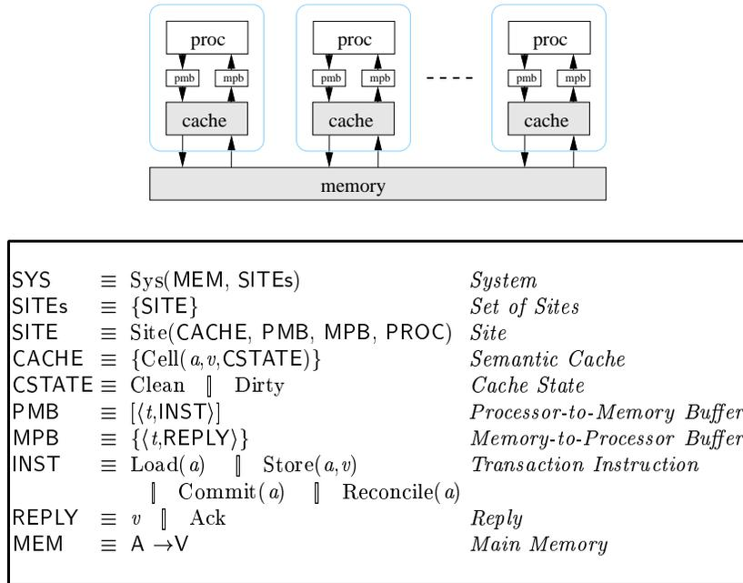
**Fig. 1.** System Configuration of CRF (omitting fences)
