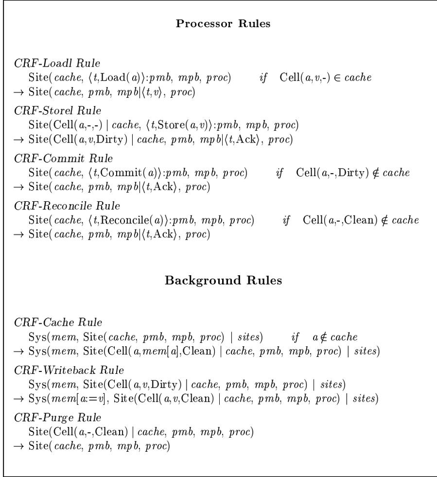
**Fig. 2.** The CRF Rules (omitting fences)
