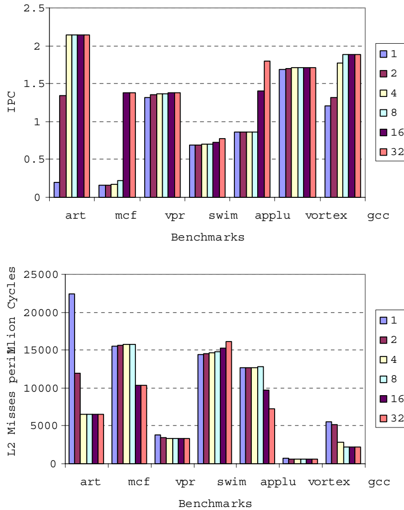
Figure 4. The L2 cache characteristics of the benchmarks used in simulations. (a) IPC as a function of L2 size. (b) The number of L2 misses per million processor cycles as a function of L2 size.
