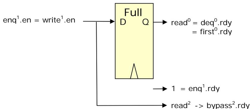
**Figure 6-3: No flow control full register ( $deq.en = deq.rdy$ )**
