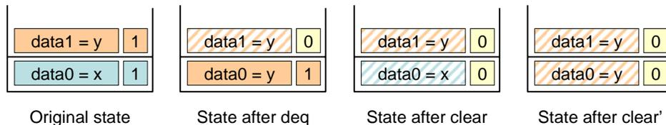
**Figure 6-12: FIFO states after deq and clear operations**
