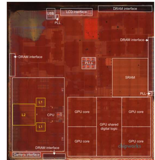
Apple A7, 28nm TSMC, 102mm 2
