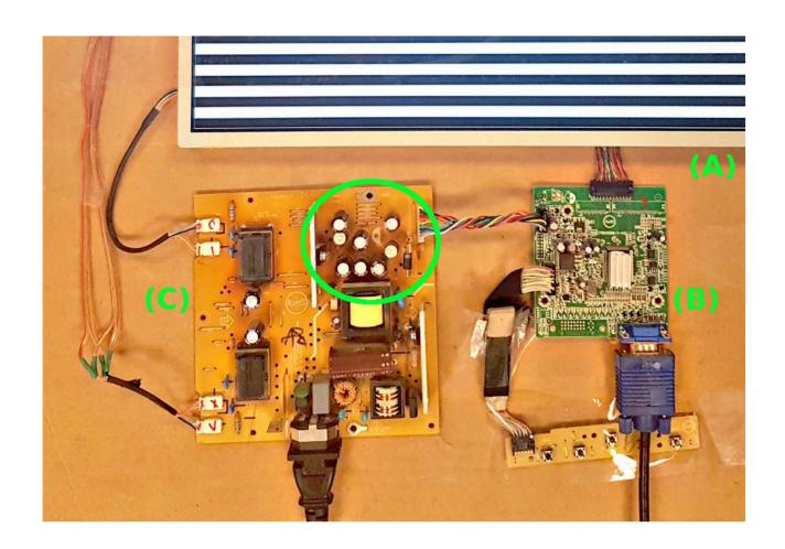
(A) is the LCD panel, (B) is the screen's digital logic and image rendering board and, (C) is the screen's power supply board.
