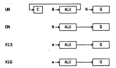
\* XI3 shifts the next "C" bit (the bit that is simultaneously being stored in "C") into the left end of the ALU result. XI6 shifts in the exclusive OR of the next "N" bit and the next "V" bit. These codes were intended for compatibility with ALU chips that were not as sophisticated as the 2903 in performing the MPY and UMPY instructions.
