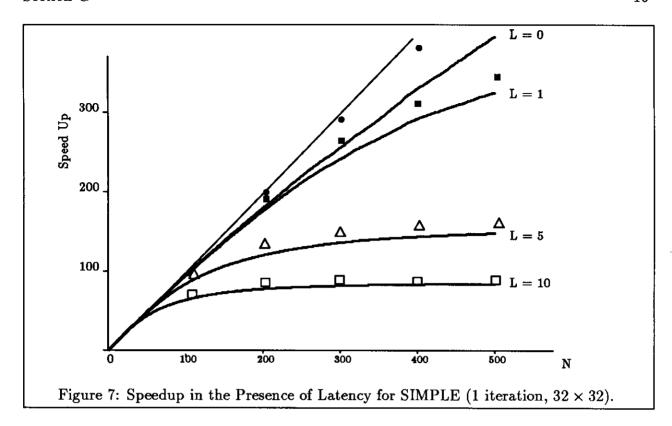
that if we do not get a near-linear speedup on a machine with, say, 50 processors and latency 10, then the fault lies with the machine, not the program. On the other hand, the program does not have sufficient parallelism to utilize a machine with 500 processors effectively.
