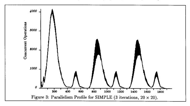
The shape of the profile for SIMPLE does not change significantly with the size of the problem.
