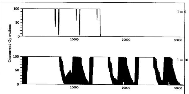
Figure 6: Effect of Latency on Parallelism Profile for SIMPLE (100 processors, 3 iterations,  $20 \times 20$ ).
