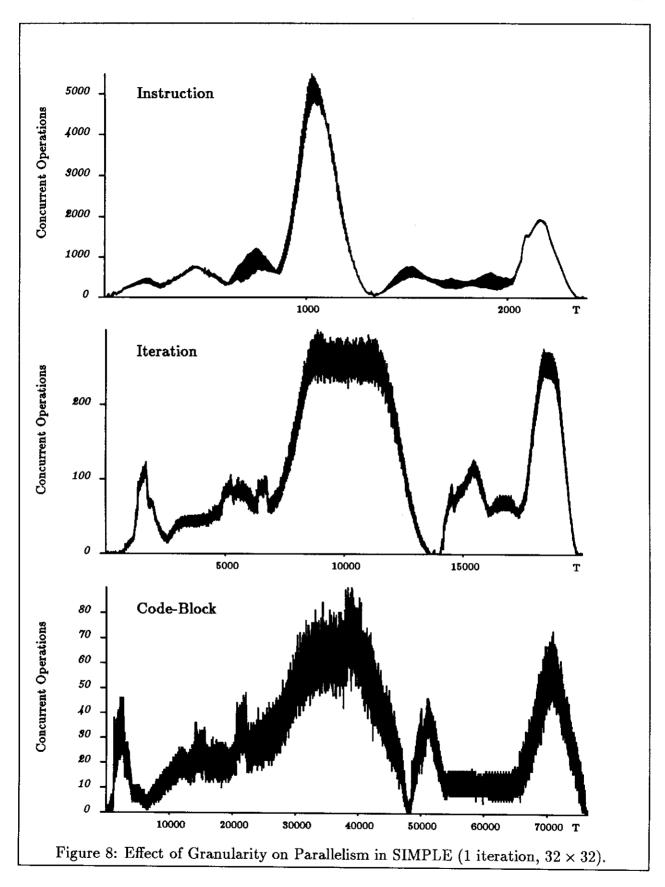
finite-processors and non-zero latency. The results show that instruction-level parallelism can keep many more processors busy.
