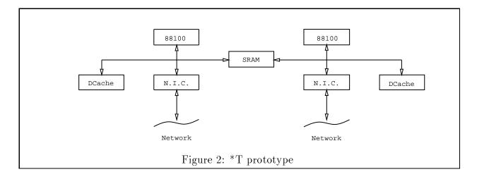
processor. Both are attached to the network via a Network Interface Chip which emulates one of 88200's data caches. The data processor sends messages directly through the N.I.C. Messages are received via another N.I.C. by the synchronization processor. Within a single node, Data and Synchronization processor communication is sped up by a dual ported SRAM which contains procedure frames and thread queue.
