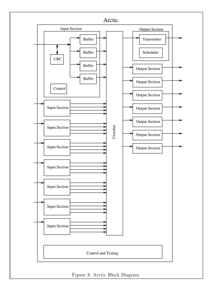
The data crossbar in Arctic has an input connected to each buffer of each input section and an output connected to each output section. Thus it can simultaneously transfer packets from any eight buffers to the eight output sections. (For example, the crossbar can simultaneously transfer 3 packets from input section 0 and 1 packet each from input sections 1 through 5.)
