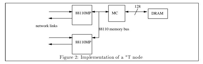
We have split the detailed design tasks with our industrial partner, Motorola. The design of the 88110MP is being done by Motorola. MIT is responsible for the design of the Arctic network router which forms the basis of the interconnection network for \*T.
