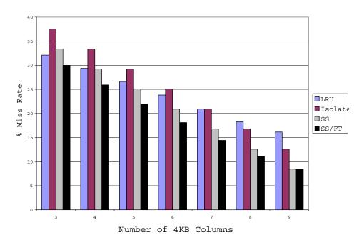
Figure 6: Miss Rates of a Synthetic Streaming Application where data is read in, looked up in a table and written out. The various mapping strategies are (i) standard LRU, no partitioning (ii) Isolated where each stream is allocated one column and the lookup table the rest of the cache (iii) Single Stream column (SS) where the two streams share the same column and the lookup table takes the rest of the cache and (iv) SS/Full Temporal, the same as (SS) but the lookup table uses the entire cache.
