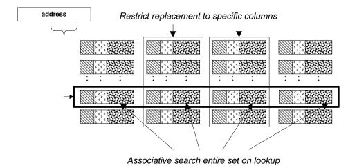
Figure 1: Basic Column Caching: Restricting Replacement in a Set-Associative Cache
