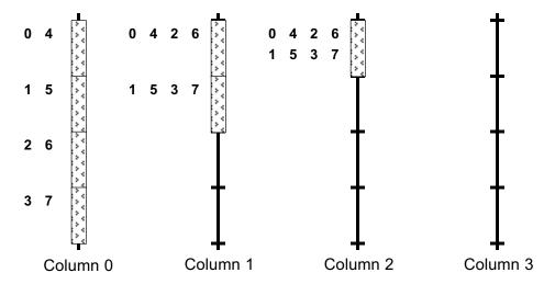
Figure 3: In column 0, pages 0 and 4 are mapped to cache page 0, pages 1 and 5 are mapped to cache page 1, pages 2 and 6 are mapped to cache page 2 and so on. Such a mapping, made possible by retargeting, allows a three column cache to vary the amount of cache space allocated to this eight page region of memory to any integer number of pages up to 7.
